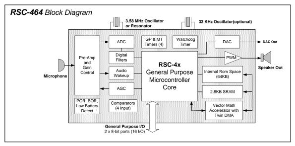
**The RSC-464** is designed to operate in tandem with the FluentChip<sup>™</sup> technology library, including speaker independent (SI), speaker dependent (SD), and speaker verification (SV) speech recognition. Combinations of these technologies may used to create applications that are rich in features. These are described below:
