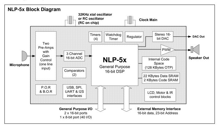
The **NLP-5x** is designed to support Hidden Markov Modeling (HMM) as well as Neural Network (NN) technologies provided in FluentChip<sup>™</sup> firmware to perform speaker independent (SI) speech recognition. A brief summary of **Speech Recognition** technologies include:
