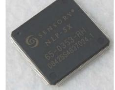
dependent and independent vocabularies, high quality stereo music, speaker verification (voice password), robotics firmware and all application code built into the NLP-5x as a single chip solution.
