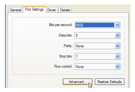
The Advanced Settings window allows you to change the COM Port number. While not necessary, you can also change the latency setting to the minimum value (1) to improve upload performance.
