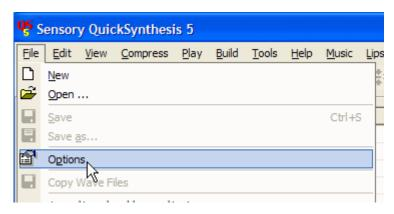
In the Options Window, select the COM port for the NLP-5x Demo/Emulation Board. To use the download feature, you will also need to select the FluentChip<sup>TM</sup> 5 for NLP-5x path. The easiest way to do this is to click on the Find button in the Options window *after* you have installed the FluentChip<sup>TM</sup> 5 Library.
