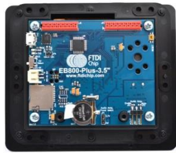
Figure 2.1 VM800P35A Module Profile 3.5" Display Version
