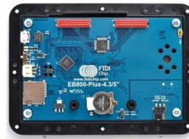
Figure 2.2 VM800P43A Module Profile 4.3" Display Version
