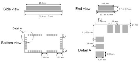
\*The pads might be slightly shorter than 1.39 mm due to PCB processing. The reduction will come from pad being pulled away from edge with up to 0.12 mm. This leaves a minimum pad lenght of 1.27 mm. The 0.1 mm distance to board edge is increase with the same number.
