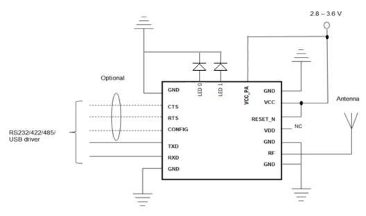
Note that the VCC\_PA pin supply the internal power amplifier only while the rest of the internal block runs on VCC. They can be connected together or separated using individual supply. For the RC1701 (low power) variant the VCC\_PA pin can be left open.
