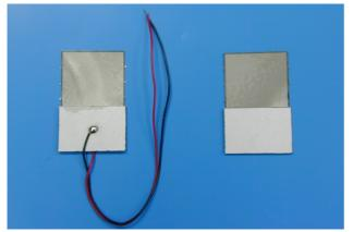
The ultrasonic vibration micro nozzle consists a piezoelectric ceramic and a metal foil, on which over thousands micro nozzles formed. Using the same principle as inkjet printer, this transducer atomizes water or liquids through a matrix of micro holes of around 7-10 µm.
