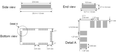
\*The pads might be slightly shorter than 1.39 mm due to PCB processing. The reduction will come from pad being pulled away from edge with up to 0.12 mm. This leaves a minimum pad lenght of 1.27 mm. The 0.1 mm distance to board edge is increase with the same pumper.
