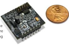
The SCOUT is designed for use in highly dynamic conditions such as high-speed gaming, remote controllers where accuracy is demanded, robotics, and limb and body tracking virtual reality...essentially any applications that require stable and repeatable tracking of physical movement.
