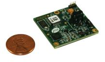
accelerometer with PNI's proprietary factory calibration and advanced field calibration algorithms to ensure absolute accuracy.
