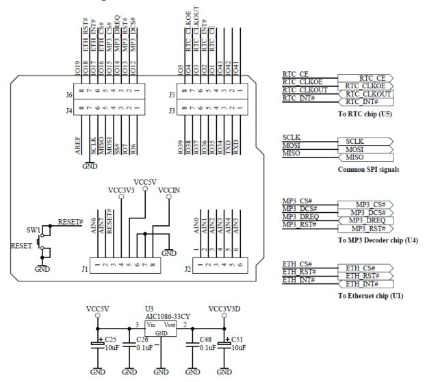
Figure 6.1 - Vinco Ethernet RTC MP3 Shield Schematic - Connectors
