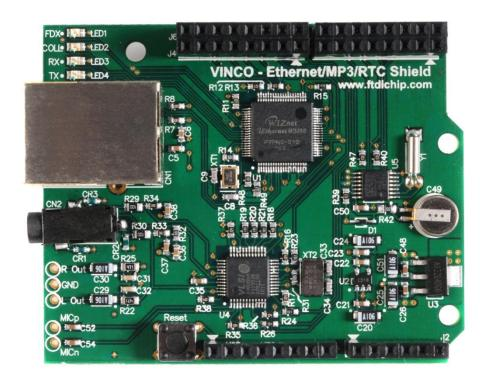
Figure 1.1 - Vinco Ethernet RTC MP3 Shield
