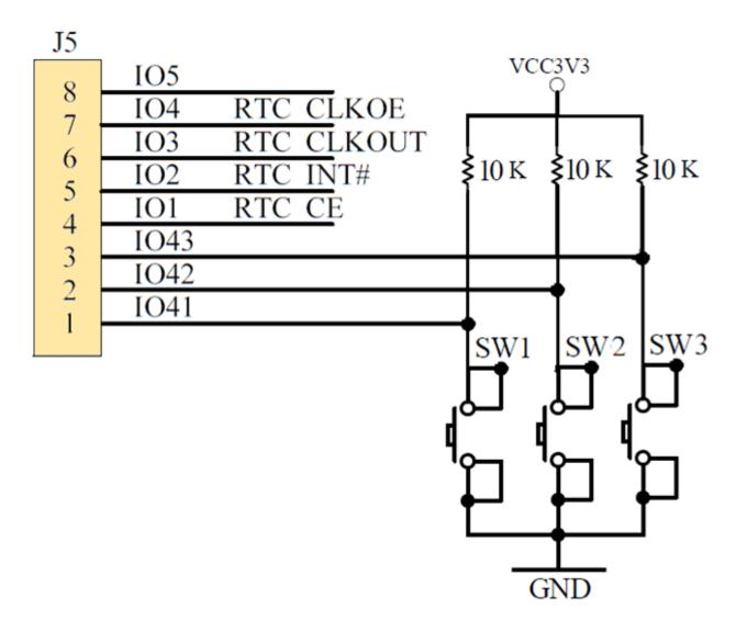
Figure 4.1 - MP3 Player Push Buttons Schematic
