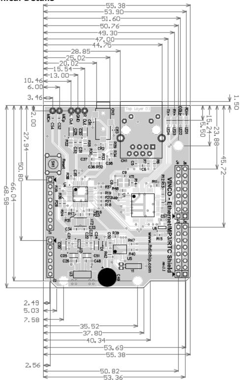
Figure 5.1 -Vinc Ethernet RTC MP3 Dimensions
