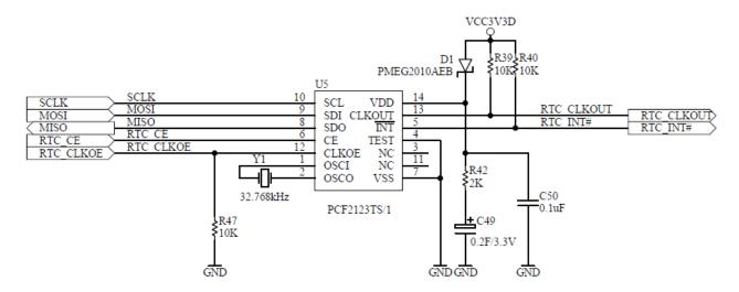
Figure 6.2 - Vinco Ethernet RTC MP3 Shield Schematic - RTC
