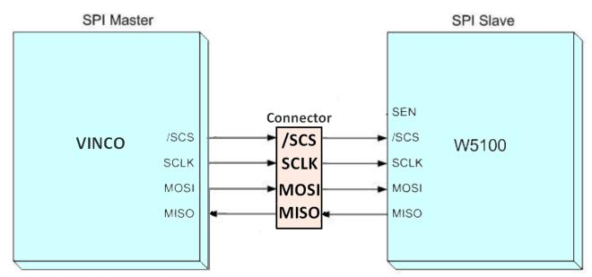
Figure 2.1 - SPI Master communicates with W5100 via the SPI bus
