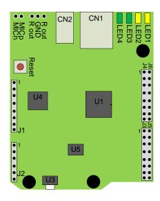
Figure 3.1 – Vinco Ethernet MP3 RTC Block Diagram
