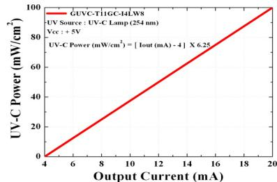
$$\begin{aligned} \text{UVC Power (mW/cm}^2\text{)} \\ = \\ (\text{Iout (mA)} - 4) \times 6.25 \end{aligned}$$
