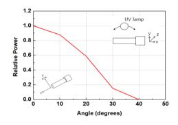
\* Position of UV lamp : parallel to z axis and perpendicular to x axis
