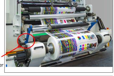
We are looking for a wear-less angle sensor. CP2HX is **not touched the sensor part and the shaft part**, so that it has been got stable **output without noise such as wear** of conductive plastic element of potentiometers.
