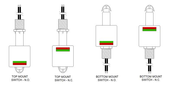
To remove and re-orient the float, gently squeeze the retainer clips at the end of the sensor and slide the float off the stem. Reinstall the float by sliding it back over the stem ensuring that it passes the clips and allows them to return to their original position.
