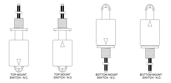
To remove and re-orient the float, gently squeeze the retainer clips at the end of the sensor and slide the float off the body. Reinstall the float by sliding it back over the stem ensuring that it passes the clips and allows them to return to their original position.
