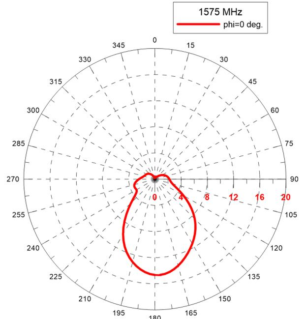
GPS RHCP Gain-Azimuth cut
