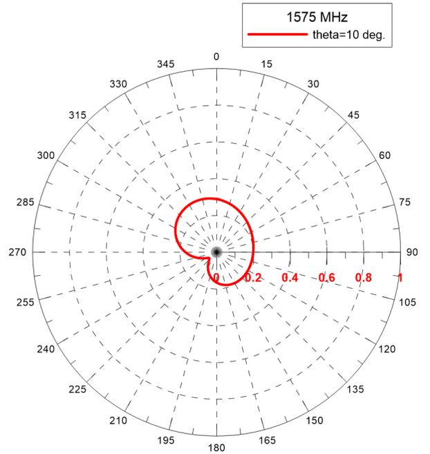
Glonass RHCP Gain-Elevation cut
