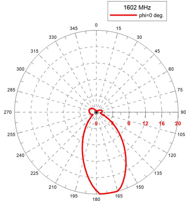
Glonass RHCP Gain-Azimuth cut
