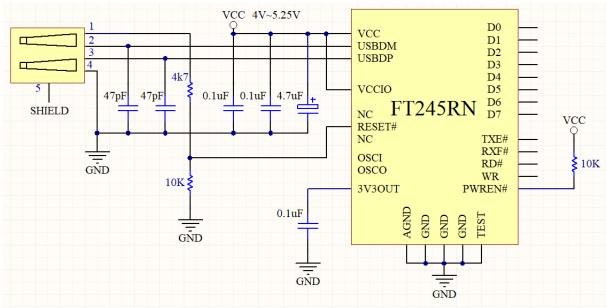
Figure 6.2 Self-Powered Configuration
