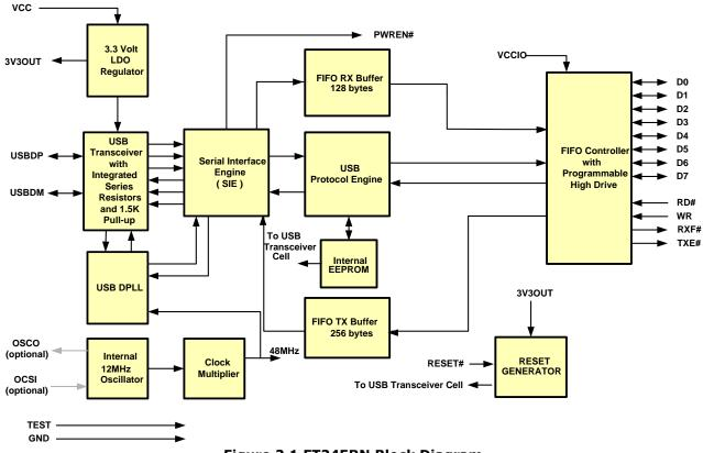
Figure 2.1 FT245RN Block Diagram
