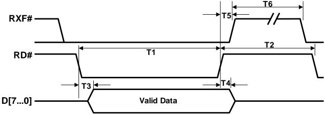
Figure 3.3 FIFO Read Cycle
