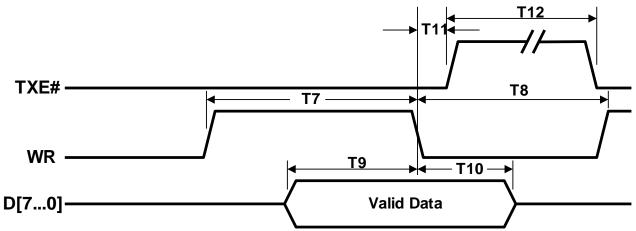
Figure 3.4 FIFO Write Cycle
