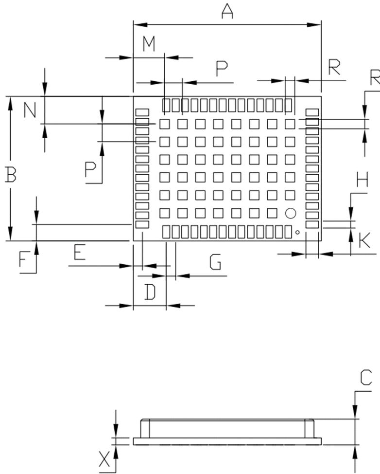
Figure 2-1 UM980 Mechanical Dimensions
