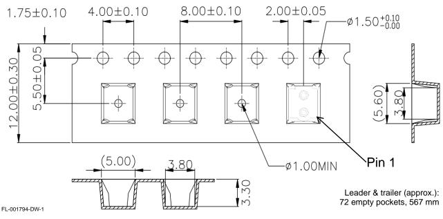
Figure 11: FLS-110-TR07 Tape Dimensions
