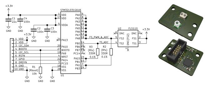
Figure 3: FLS110-STM32 reference design schematic and module implementation
