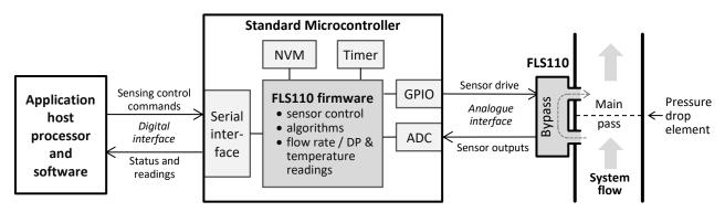
Figure 1: Example of an FLS110 flow sensing solution with dedicated microcontroller
