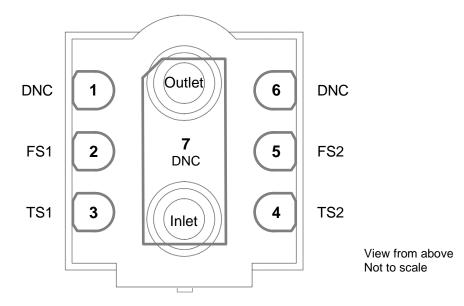
Figure 8: Pin and port positions
