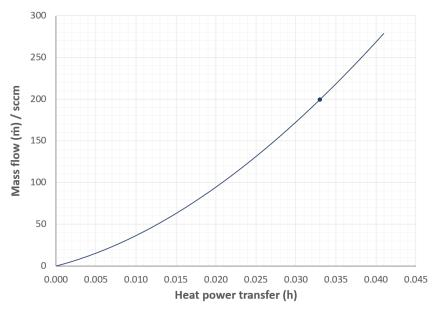
Figure 6: Typical relationship between mass flow (m) through the FLS110 and heat power transfer (h)
